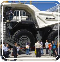
The Liebherr T 282C is the ultimate monster in automotive at the moment! It is the size of a house and its engine gives 3650hp. It weighs 252tons and can carry up to 400tons.
